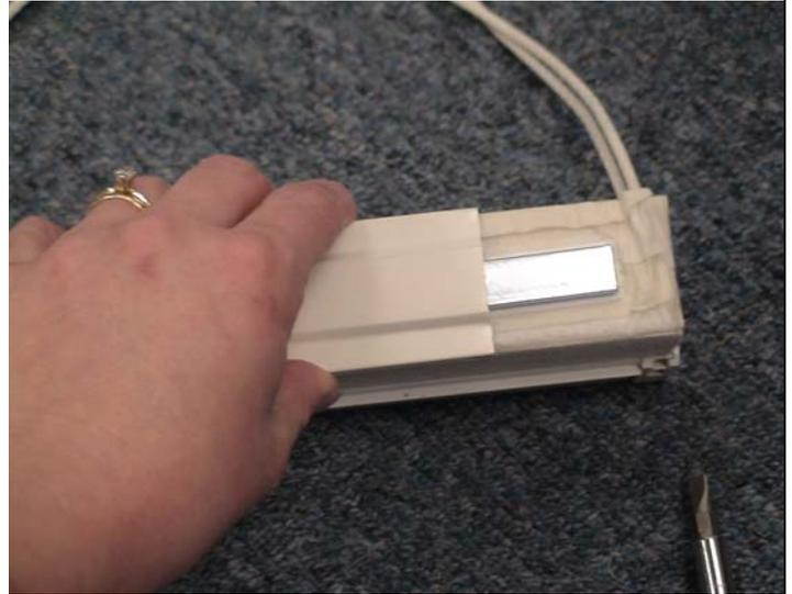
10. Locate the cord on the side of the shade that is lower. Retie knot in cord so the shade is even in length.
