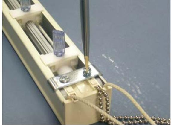
7. Insert the new control mechanism into the open end of the headrail. Insert the pinion rod securely into the center of the control mechanism housing. Make sure the cords are placed over the wheels and in the grooves and push the control mechanism until it is flush with the end of the headrail. Tighten screws.
