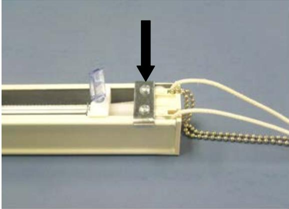
6. Loosen screws with a #2 Phillips head screwdriver. After screws have been loosened, pull control mechanism off the end of the headrail.
