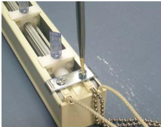
8. To ensure control mechanism has been installed correctly, rotate stems open and closed several times using chain and traverse carriers by pulling on traverse cord to test operation.
